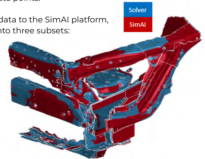
A comparison between Ansys SimAI software and solver predictions of a bumper’s deformed shape at a given time show the SimAI model predictions to be reasonably accurate.
